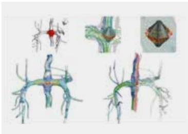
Images from the computational surgical implantation and high-fidelity blood flow simulation of the chronic pump in a patient-specific Fontan circulation showing blood vessel and pump geometry together with complex flow patterns, structures and particle tracks.
